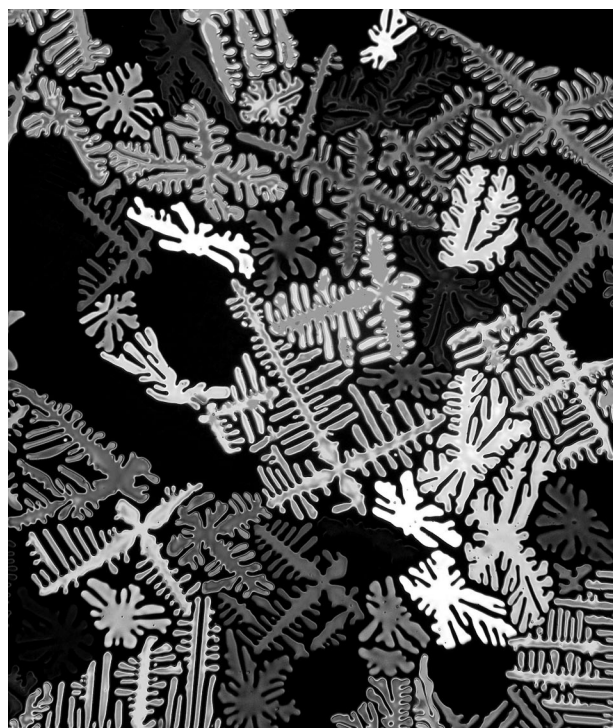
Figure 2. POM image of the columnar phase of 2c at 130 °C (crossed polarizers; 500× magnification).
